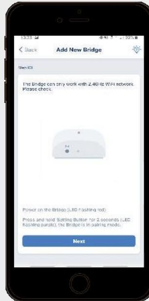
With bridge powered on, press And hold setting button for 2s (LED flashes purple for pairing), The bridge is in pairing mode
